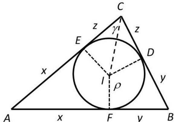
$$\sphericalangle ECI = \frac{1}{2} \cdot \gamma, \sphericalangle CIE = 90^\circ, |\overline{EI}| = \rho$$
